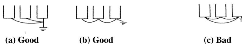
Figure 3-6 Grounding examples: multiple drives
